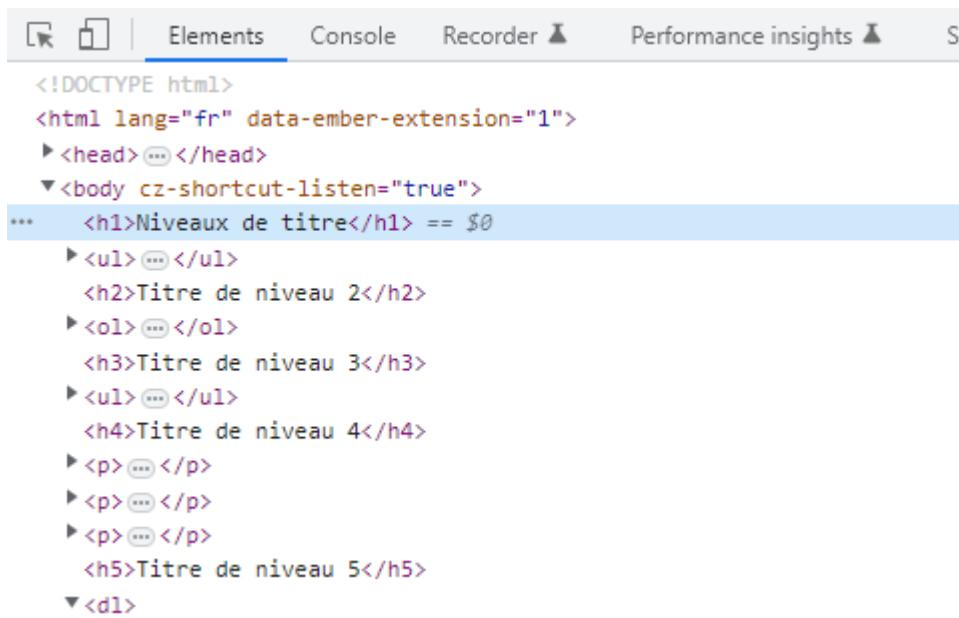
The screenshot shows the Chrome DevTools interface with the 'Elements' tab selected. The DOM tree is displayed, starting with the root <!DOCTYPE html>. The tree structure includes a <head> element, a <body> element with the attribute 'cz-shortcut-listen="true"', and several child nodes: <h1>, <ul>, <h2>, <ol>, <h3>, <ul>, <h4>, <p>, <p>, <p>, <h5>, and a <d1> element. The <h1> node is highlighted with a blue background.
